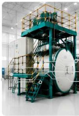
VACUUM CASTING PLANT
